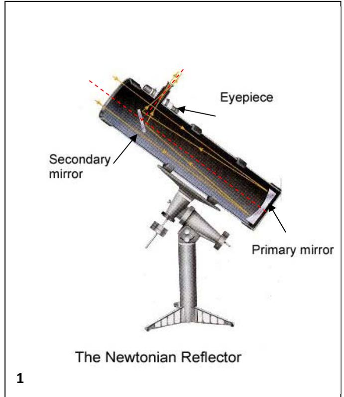
as shown in the picture. This makes it form a "Real Image" of a distant object at its "Focal Plane". The eyepiece is like an ordinary magnifying glass to enable you to examine this real image closely. Figure 2 shows the top end of the optics, *as properly adjusted*. **The telescope will only give sharp images everything is properly adjusted!**
